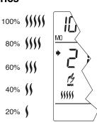
To see this process, the display shows, in real time, the percentage of power applied to the electric heating system.
