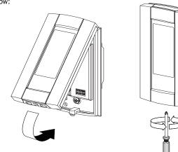
To remove the face plate from the power base, invert steps.
