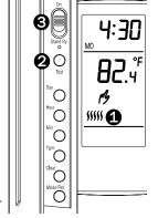
**3.** When successful, reset FloorStat (On/Standby) to power the heating system.
