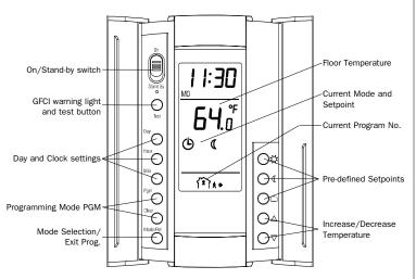
**NOTE:** The 500650 face plate must be mounted on a PB112 Series Power Base.
